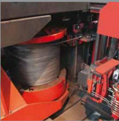
The vertical automatic spooler type SirioStar is the highest innovative system used for the production of compact smooth or reinforcing wire coils with 5 ton maximum weight.
