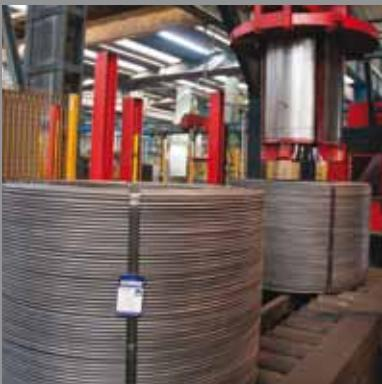
SirioStar is the most flexible spooler that produces compact wire coils or fixed spools starting and ending the winding either from the lower or the upper spool flange.
